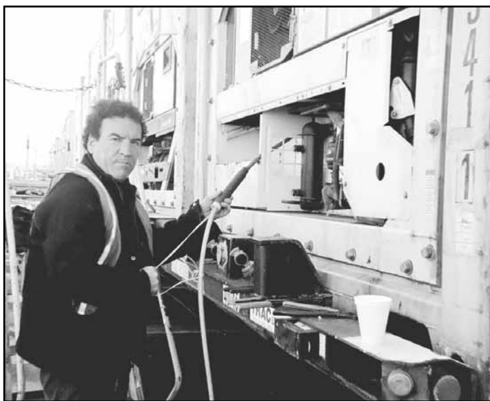
Shore mechanic Bruce Botai, #3737, splicing a reefer container power cord at the APL Global Gateway Central facility in Oakland.
